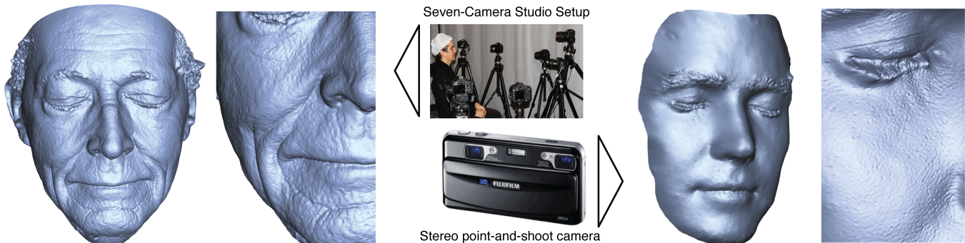
Figure 1: Left: Face model captured using a seven camera studio setup; Center: capture systems; Right: Face model captured using consumer binocular-stereo camera. Facial geometry in all figures is best viewed in the electronic version.
